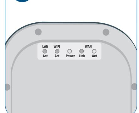
At power-up, the Power LED and the WAN Act LED illuminate and the WAN Act begins blinking. When you confirm a network connection, tighten the clamps to complete attachment of the SkyAccess DualBand to the mount.
