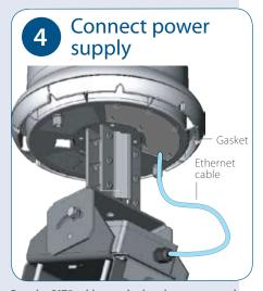
Run the CAT5 cable attached to the power supply through the gasket and plug it into the RJ-45 port on the SkyExtender base.
