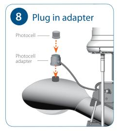
Connect the photocell adapter to the photocell socket then reconnect the photocell by plugging it into the receptacle on top of the adapter. Make sure the excess photocell adapter cable is tightly wrapped and secured—the space under the mount stand will accommodate the coiled cable.
