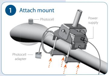
Use the provided bolts and clamps to attach the mounting bracket to the pole. Position the mount so that cable terminating in a photocell adapter is oriented towards the photocell—usually attached to the top of the street lamp.
