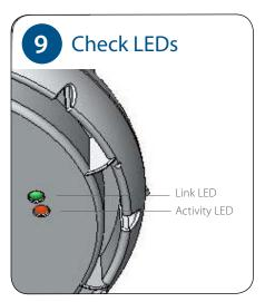
As the device powers up, check the LEDs on the base of the SkyExtender. When both LED lights are lit and steady, the device is successfully connected to the network.
