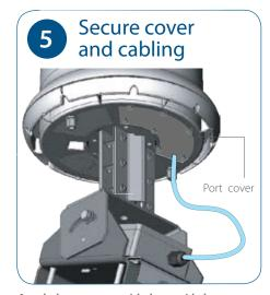
Attach the port cover with the provided screws, making sure the CAT5 cable passes through the cutout. Use cable ties to provide appropriate strain relief for cabling.
