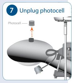
Locate the photocell on the light pole(usually located on top of the lumiere) and remove it from the socket.
