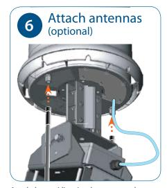
Attach the omnidirectional antennas to the connectors on the base of the SkyExtender DualBand or SkyExtender TriBand.
