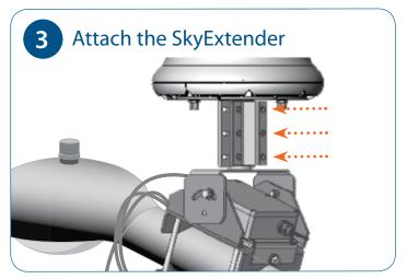
Use the provided mounting bracket to attach the SkyExtender to the pole mount. Note: If you're installing a SkyExtender DualBand or SkyExtender TriBand, rotate the device to ensure there is ample room for the omnidirectional antennas to clear the mount stand.
