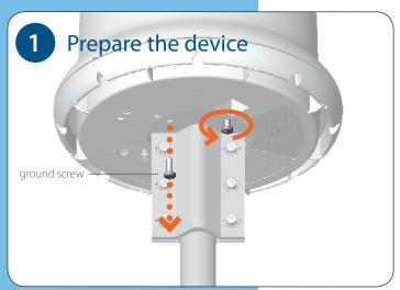
Remove the ground screw from the base of the device, and then loosen (but do not remove) the screw on the same side of the bracket as the ground screw.
