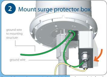
Reattach the ground screw, running it through the lug on the ground wire from the surge protector box, the mounting bracket on the box, and the lug on the ground wire from the SkyPilot device. Pivot the box into place and tighten the screws.
