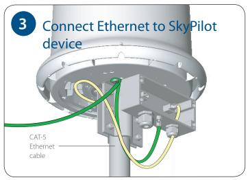
Remove the cable cover plate from the SkyGateway/SkyExtender. Remove the cover plate from the surge protector box. Plug the Ethernet cable extending from the surge protector box into the Ethernet connector on the SkyPilot device.
