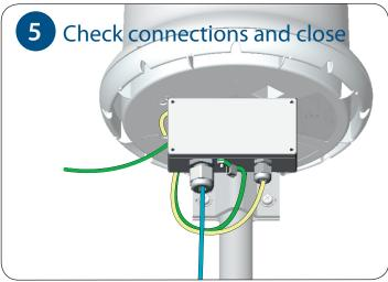
Route the CAT-5 shielded Ethernet cable from the PoE Injector through the cable Check the connections and reattach the surge protector box cover plate. seal gasket. Separate the drain wire from the cable and plug the cable into the connector labeled LINE. Attach the drain wire to the provided crimp lug and push the lug onto the tab extending from the internal ground bolt.
