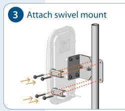
Use the original mounting brackets with the provided 2 1/4" panhead screws and washers to attach the SkyConnector with tilt assembly to a pole. (Diameter of pole must not exceed 1 3/8".)
