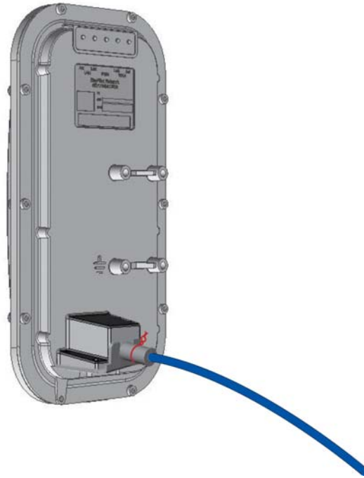
Figure 3-3. Attaching tie wraps to the gasket neck
