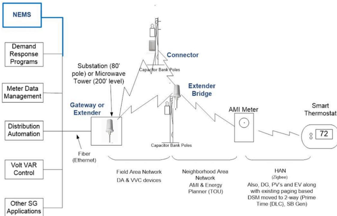
*Utility X plans to implement its Smart Grid in phases, beginning with Distribution Automation and Volt/VAR Control.*
